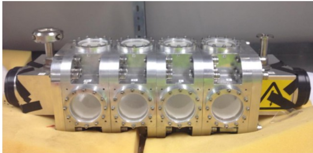
Prototype target from Max-Lab with external PMT readout (in Mainz)
