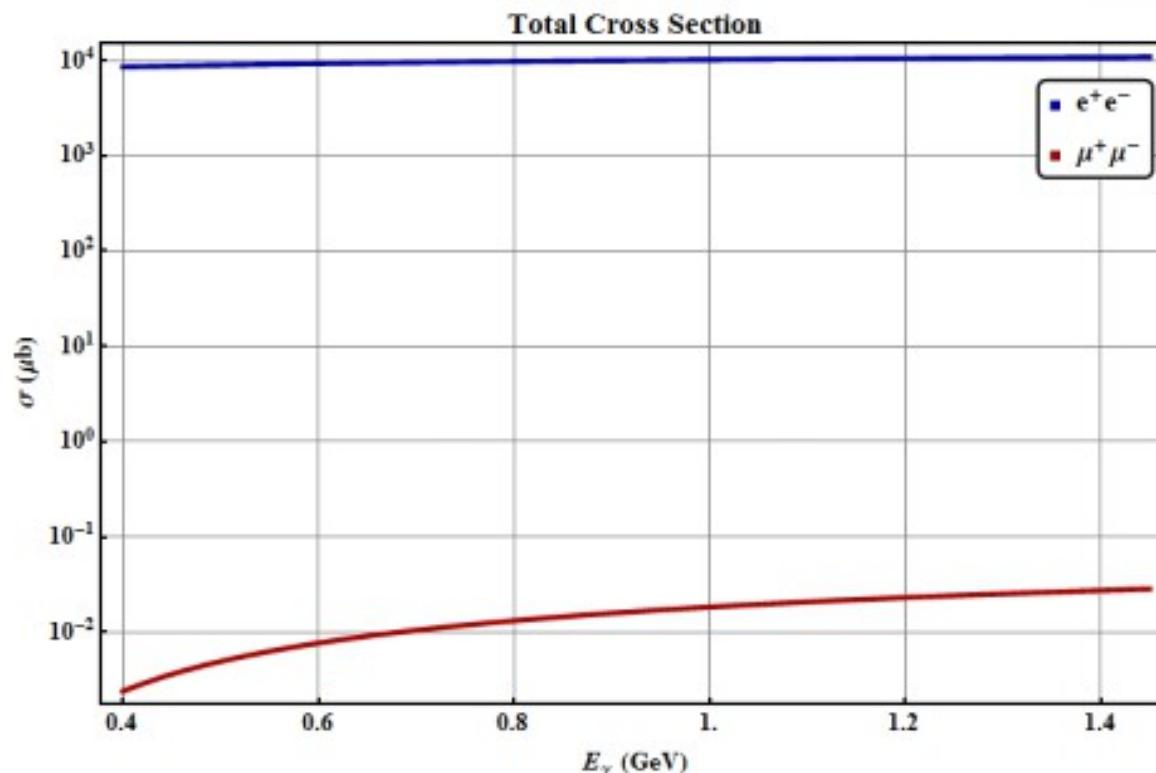
BH- $e\bar{e}$  (blue) and BH- $\mu\bar{\mu}$  (red) cross section as function of beam energy
